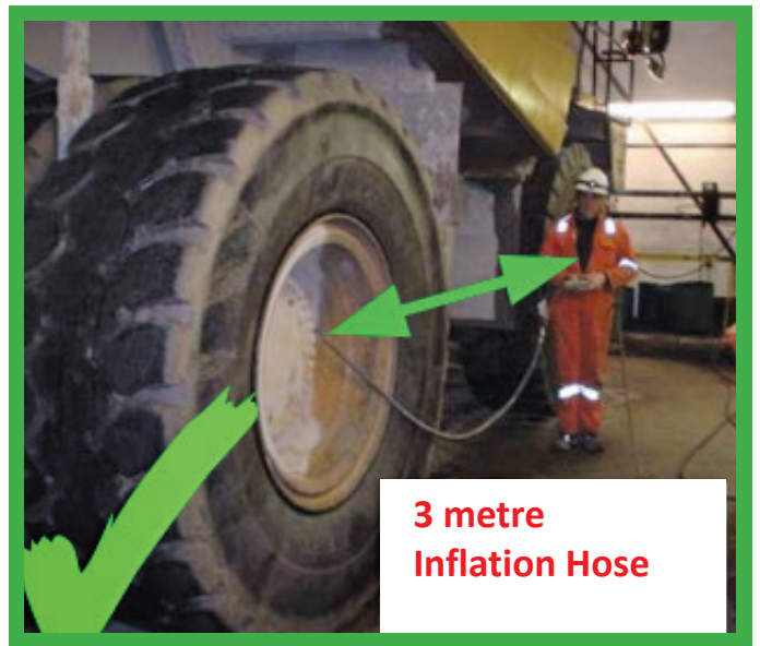
Best Practice example: To eliminate the risk of over inflation of tyres, tyre pressure is inputted remotely into a control unit. The 15 metre airline is then fitted to the vehicle (away from the control unit ) and a preset air pressure is used to inflate the tyre. Access to the control is restricted as users require access codes.
