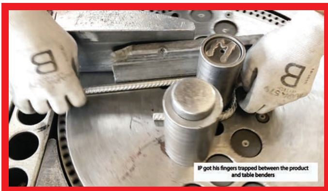
2020 Accident involving a bending machine: IP got his fingers trapped between the product and table benders.
