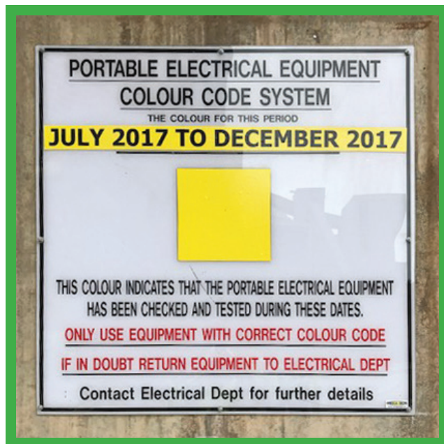
Instructions for all users of portable electrical equipment to only use equipment with correct colour code tag for that period.
