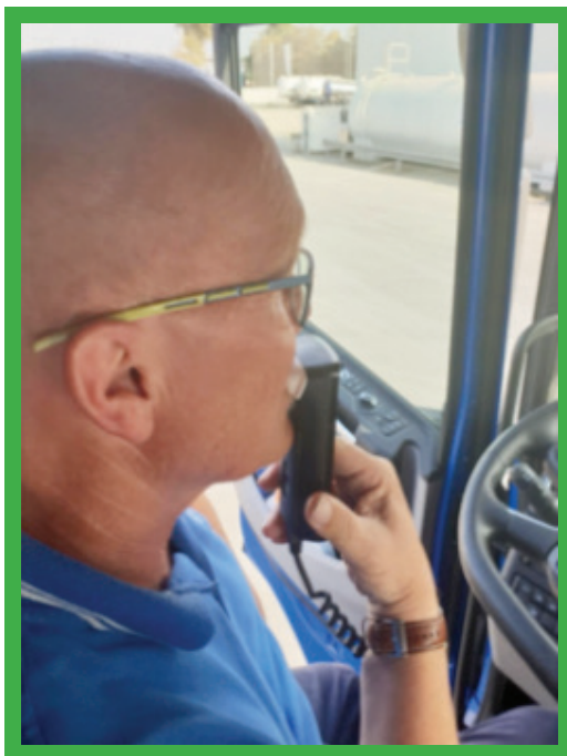
An alcohol tester designed into the truck ignition system – driver must give a negative result for truck to start.
