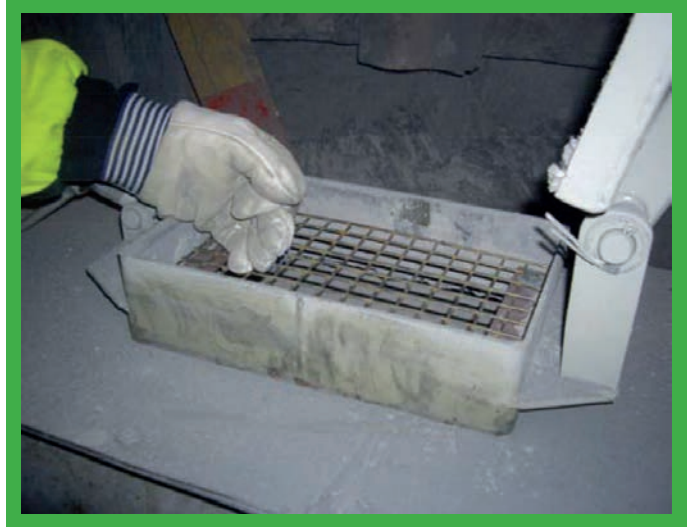
Inspection hatch (with secured grid) on a screw conveyor.
