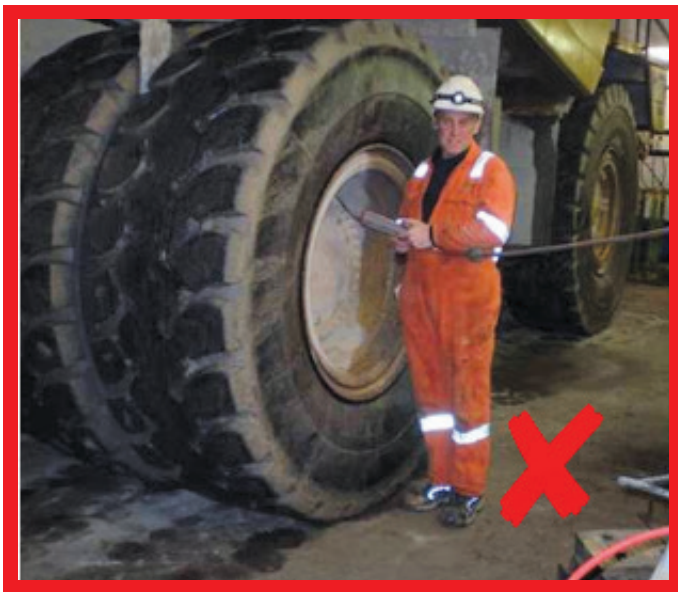
Best Practice example: To eliminate the risk of over inflation of tyres, tyre pressure is inputted remotely into a control unit. The 15 metre airline is then fitted to the vehicle (away from the control unit ) and a preset air pressure is used to inflate the tyre. Access to the control is restricted as users require access codes.
