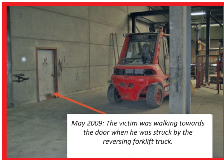
Group Fatal Accident - Case Study: Contract fitter struck and killed by a Forklift unit.
