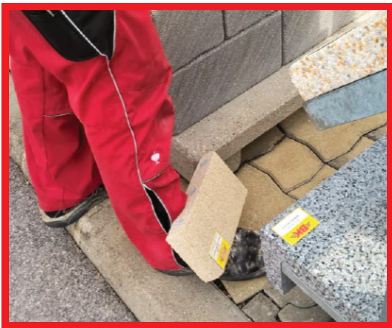
August 2017 accident: contractor suffered serious foot injury after blocks landed on area behind the steel toe cap shoe and struck the area that would have been covered by a metatarsal shoe or boot.
