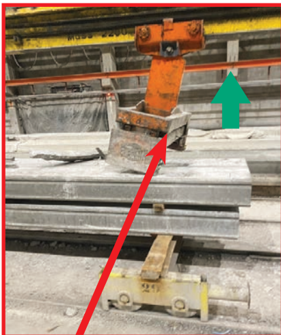
When the slab was lowered into position - the operator released the grabs / clamp and lifted the clamps higher upward to move them away from the next task.
